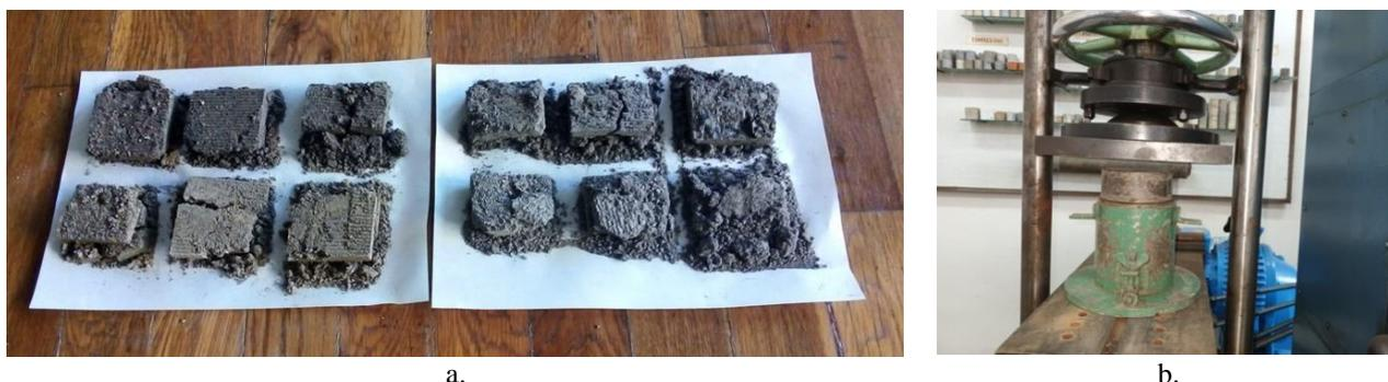
Fig. 4. Laboratory tests; a. Rock samples subjected to direct shearing tests; b. Sample subjected to an overload corresponding to the natural loading determined by the lithological column in order to determine the volumetric weight of the rocks
