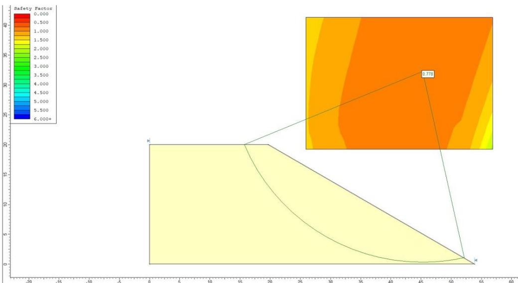
Fig. 6. Stability analysis for the dump step having  $h = 20 \text{ m}$  and  $\alpha = 30^\circ$  ( $F_s = 0.778$ )
