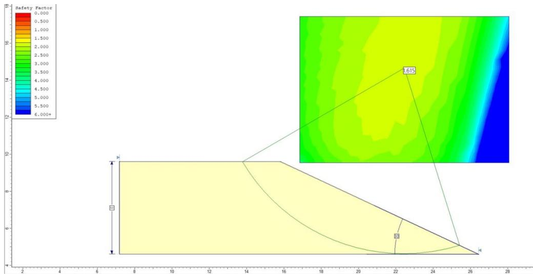
Fig. 5. Stability analysis for the dump step having  $h = 5 \text{ m}$  and  $\alpha = 30^\circ$  ( $F_s = 1.615$ )
