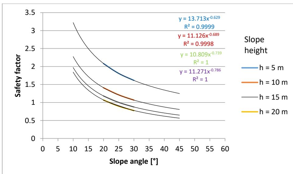
Fig. 8. Variation of the safety factor as a function of the slope angle at different values of the slope height (power function)
