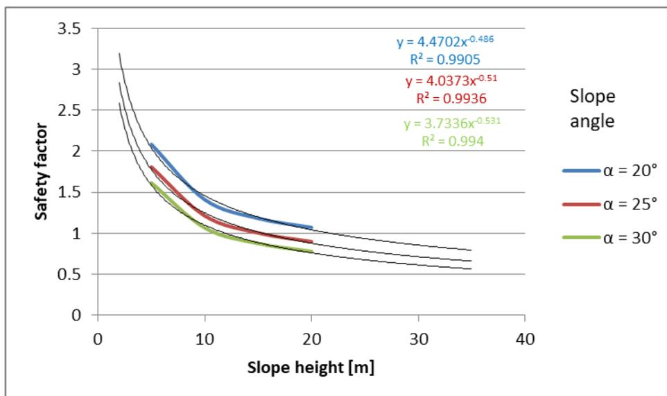
Fig. 7. Variation of the safety factor as a function of the slope height at different values of the slope angle (power function)
